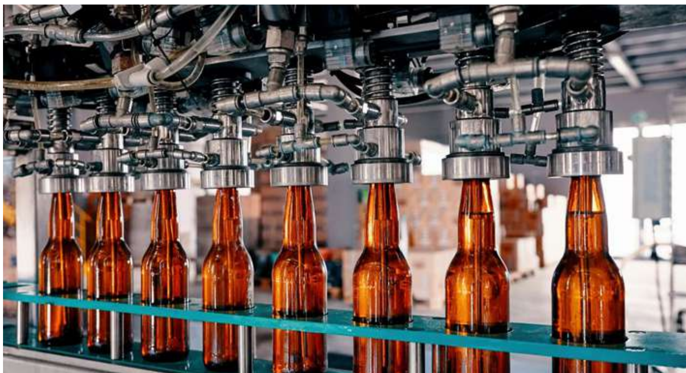
Beer bottles filling on the conveyor belt in the brewery factory. SOURCE | SHUTTERSTOCK / CAGKAN SAYIN
