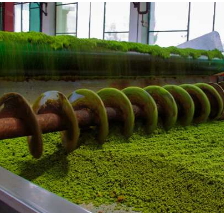
CTC (crush, tear & curl) Plant in a black tea manufacturing factory SOURCE | SHUTTERSTOCK / ANIL VARMA
